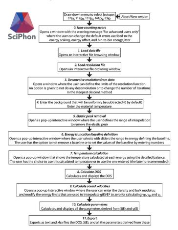
Figure 1 Flowchart of the *SciPhon Mathematica* package. Fig. 3 shows how these actions are implemented through GUI display panels. See text for details.
