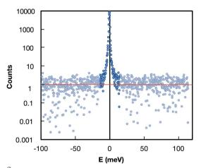
Figure 2 Example of the resolution function measured in the nuclear forward-scattering channel. The FWMH is  $\sim\!1$  meV. The intensity decreases by four orders of magnitude in the first  $\pm15$  meV. Beyond that, the measured counts are below baseline level. Before further processing, the baseline counts (in red here) are subtracted form the signal and the spectrum is truncated to eliminate the low- and high-energy tails where the signal is below baseline (here beyond  $\sim\!\pm15$  meV).
