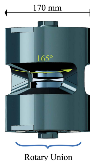
Figure 8 Schematic of the new design of a PE press optimized for in situ imaging. This press is significantly smaller (170 mm diameter) and presents a wider opening of 165^\circ which will allow a higher quality of imaging. A rotary union is used for the water-cooling system as well as the electrical wiring. This will allow acquisition upon continuous rotation at a fixed pressure reducing the acquisition time of a tomogram.
