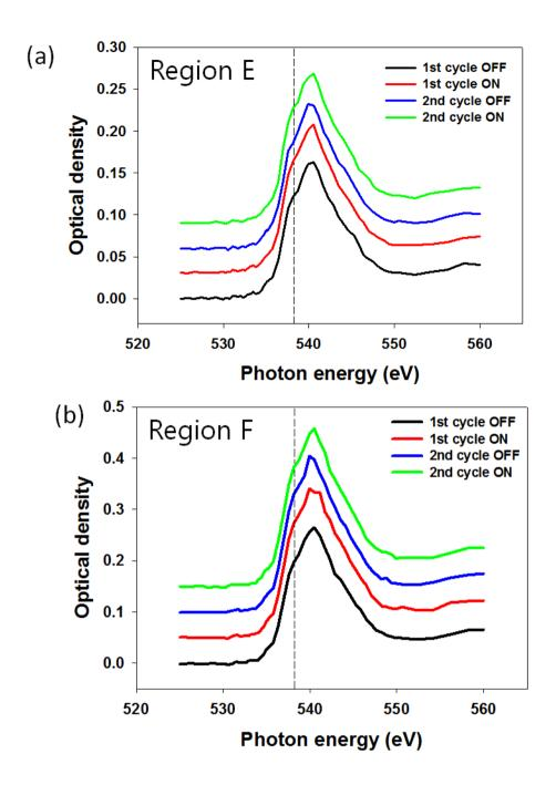
Figure S1 O K-edge XANES spectra of ReRAM in region E (a) and region F (b).
