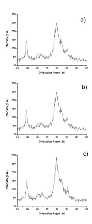
**Figure 1** X-ray diffractograms of Pb-HA powders: a): PbHA\_1; b): PbHA\_2; c): PbHA\_3 showing the (002) reflexes (at about 25.87 ° 2 Theta) and the (211), (112) and (300) reflexes (between about 31 ° and 33 ° 2 Theta) which are not angular resolved because of the peak broadening due to small crystallite sizes.
