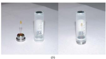
**Figure 2** (*a*) The standard sample holder and its vial standardized by SPINE. (*b*) A modified sample holder for non-frozen samples with a capillary instead of a cryo-pin.
