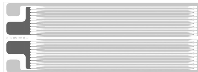
Figure 1 Drawing of the electrode pattern used for this detector.
