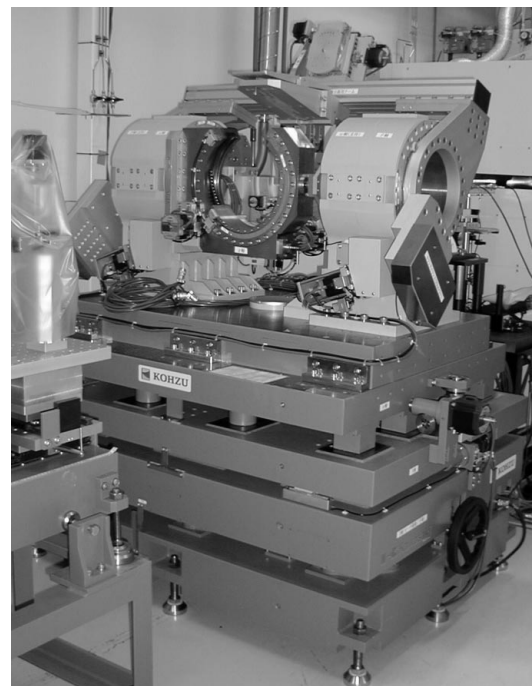
Figure 1 Photograph of the X-ray diffractometer at SPring-8 BL24XU.
