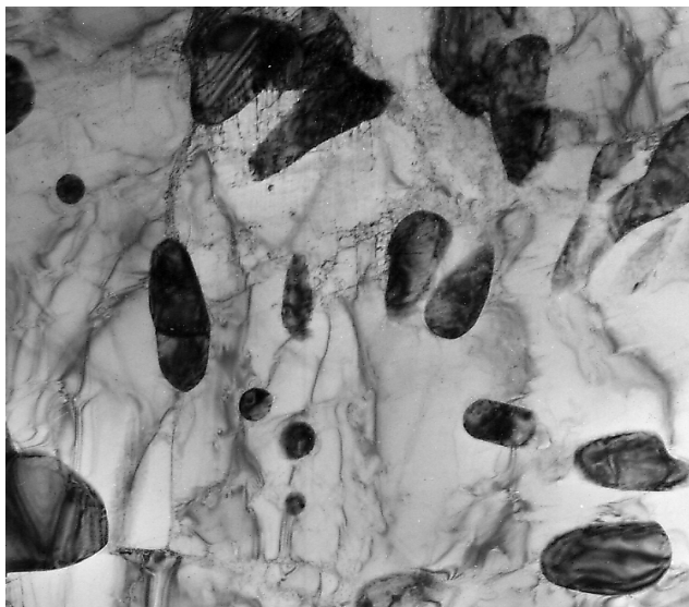
Figure 2 Microstructure of the carbon steel U15 pearlite obtained by quenching from 1050°C followed by annealing at 500°C for 2 min, cooling to room temperature and additional annealing at 700°C for 20h (regime 2)
