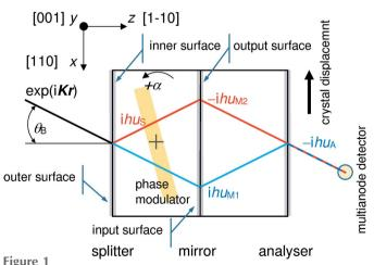
X-ray phase-contrast topography. The X-ray paths are drawn in red (RRT path) and blue (TRR path). The Bragg angle is out of scale. The phase delay of each reflection is given. The X-ray crossings with the mirror are spaced by 4 mm. Adapted from Massa *et al.* (2020*a*).
