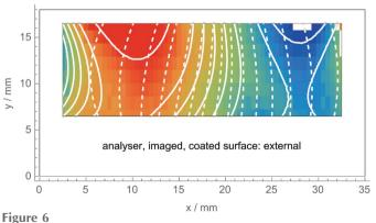
Top: predicted observation of the displacement field when the outer side of the splitter or the analyser is coated. Middle and bottom: observed displacements. The colour scale is from -110 pm (blue) to 110 pm (red). White lines are contours of constant displacement (solid) and the diffracting planes with displacements magnified (dashed). The white pixels indicate outliers excluded from the analysis.
