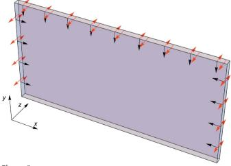
Figure 2 Surface stress modelling by forces per unit length applied orthogonally to edges and lying in the crystal surfaces. Black: forces acting on the coated z = 0 mm surface. Red: forces acting on the crystal rim. The boundary conditions specify a displacement field equal to zero at the bottom, y = 0 mm, surface.
