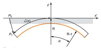
Figure 9 Geometry of the bent crystal; y' = const. section. The axis x is normal to the diffracting planes, and the axis z is normal to the crystal surfaces. The orange line indicates the Cu coating. The rear surface lies in the neutral plane, z' = 0.
