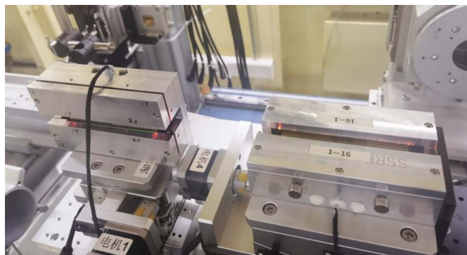
Figure 5 Photograph of the KB focusing system. The left HFM is the deformable mirror with linearly changing thickness and the right mirror is the VFM with a fixed elliptical shape.
