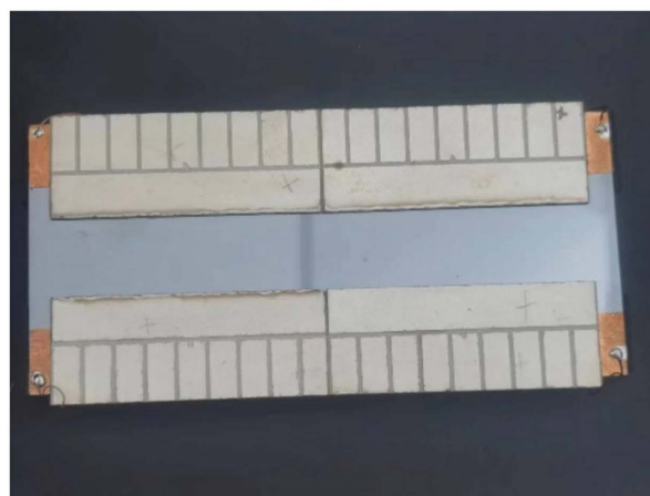
Figure 2 Diagram of the focusing mirror and arrangement of the piezoelectric ceramics. (a) The linearly changing thickness of the prototype silicon mirror is shown in a side view. Two long actuators (19 and 20) near the optical area are used to adjust the overall shape of the mirror to an ellipse. The small actuators 1–18 are used to adjust the overall shape and compensate the figure error of the elliptic surface to improve the focusing performance of this mirror. (b) Corresponding photograph of the prototype mirror.
