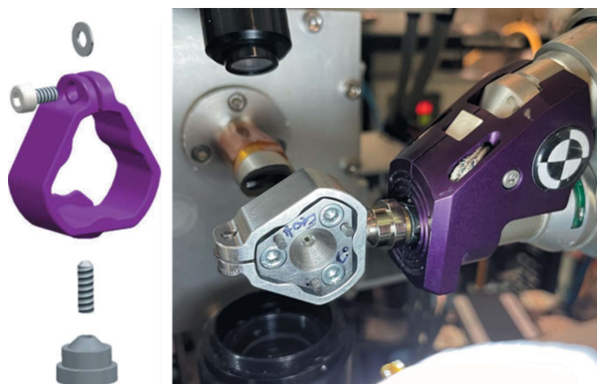
Figure 2 MMB magnetic base-cell holder clamp design and MMB cell mounted onto the MX1 beamline at the Australian Synchrotron.
