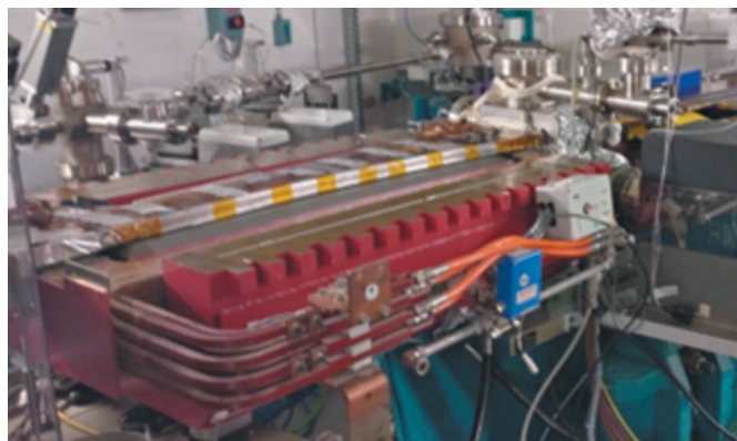
Figure 15 The Superbend vacuum vessel installed temporarily inside the standard electromagnetic dipole and equipped with heating films. The upper yoke of the electromagnetic dipole is not yet back in place in the photograph.
