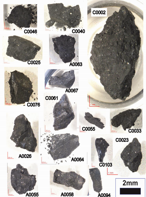
The 17 coarse Ryugu samples used in this study. The images are shown on approximately the same scale. Each panel is labeled with the sample identification number. Mossbauer spectroscopy work was performed on samples A0026 and C0061
