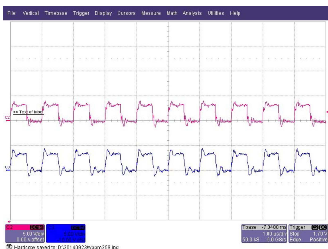
Figure 4 Two channels of hardware trigger signals: one is for the ADC, the other is for the scaler.
