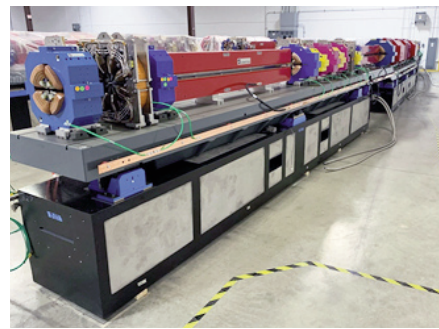
Fully assembled mock-up of one MBA-lattice storage ring sector on a plinth.
