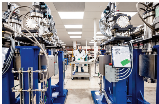
Two of the new front-end table systems under construction in the APS-U offsite building.
