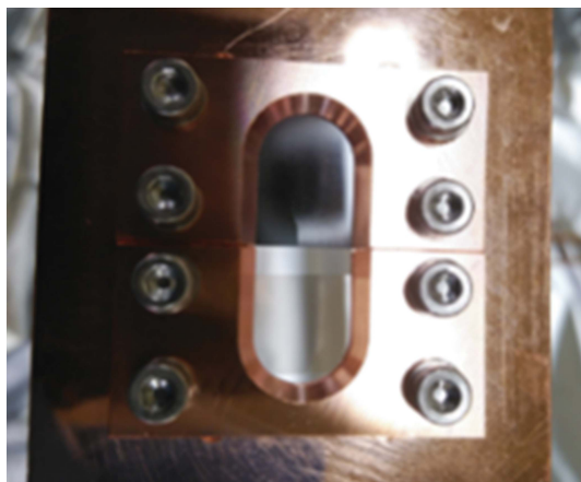
Figure 2 Installation of a diamond film on the copper block cooling system.
