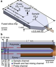
CAD-renderings of microfluidic mixer. (a) Isometric view of fused silica chip-polyimide capillary subassembly with key dimensions labeled. The three inlets to the chip are labeled. (b) Cross-sectional view at the location of the dashed line in (a). The three channels inside of the fused silica chip are highlighted for clarity.
