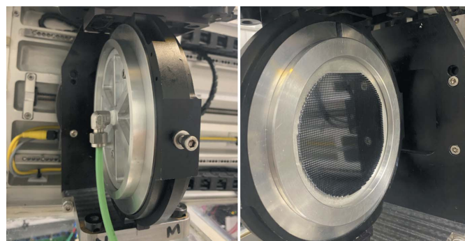
Figure 2 Front and back views of the analyzer mounted inside the spectrometer at sector 27 at the APS.
