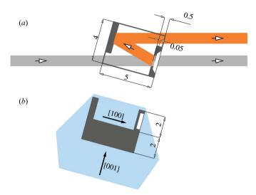
Figure 4 Schematic diagrams of the (800) diamond channel-cut crystal monochromator for 14.4 keV X-rays (black). The channel cut is machined from an as-grown cubo-octahedral diamond crystal stone (light blue). Shown are (a) top and (b) side views with dimensions in millimetres. The propagation paths of the X-ray beams with a 1 mm<sup>2</sup> cross section are shown in panel (a).
