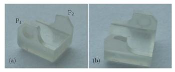
Figure 6 Photographs of the (620) channel-cut crystal after annealing.
