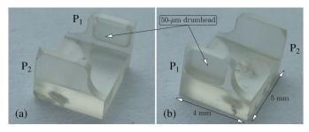
Figure 7 Photographs of the best-quality (800) channel-cut monochromator crystal (third iteration) after annealing. Note the optimized rectangular shape of the drumhead  $\sim$ 2 mm  $\times$  1.4 mm in size and 50  $\pm$  5 µm thick.
