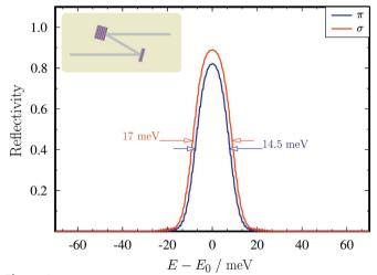
Figure 2 Diamond crystal reflectivity for X-rays in two successive 800 Bragg reflections calculated as a function of photon energy E with a central energy,  $E_0$  = 14.4125 keV, corresponding to the nuclear resonance of <sup>57</sup>Fe. The Bragg angle is  $\theta$  = 74.7207°. The photon energy dependences are calculated for two possible X-ray polarization states,  $\pi$  and  $\sigma$ .
