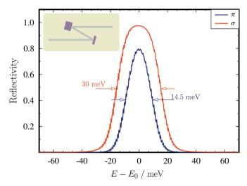
Figure 3 Diamond crystal reflectivity for X-rays in two successive 620 Bragg reflections calculated as a function of photon energy E with a central energy,  $E_0 = 12.4 \, \mathrm{keV}$ , corresponding to the nuclear resonance in  $^{45}\mathrm{Sc}$ . The Bragg angle is  $62.424^\circ$ .
