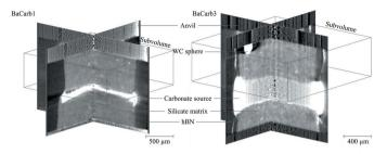
Figure 2 Tomography cross sections with studied subvolume representation. The illustrated cross sections are from the last CT images of cycle 3 for both samples BaCarb1 and BaCarb3 (see Table 1 for more details).
