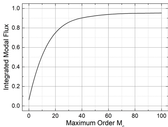
Figure 6 Integrated modal flux \hat{F} as a function of the maximum order of the coherent modes M_c .
