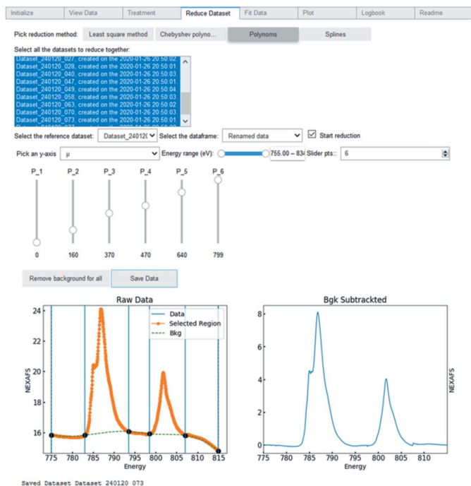
Figure 9 Application of the polynomial curves method to remove the background from a representative NEXAFS spectrum at the Co L -edge (orange points, left panel) containing both the L_2 - and L_3 -edges. After having selected the working energy range and the number of spectral points needed to generate the background function, the user can move them along the spectral profile through sliders while simultaneously observing their effect on the background-subtracted spectrum (blue curve, right panel).
