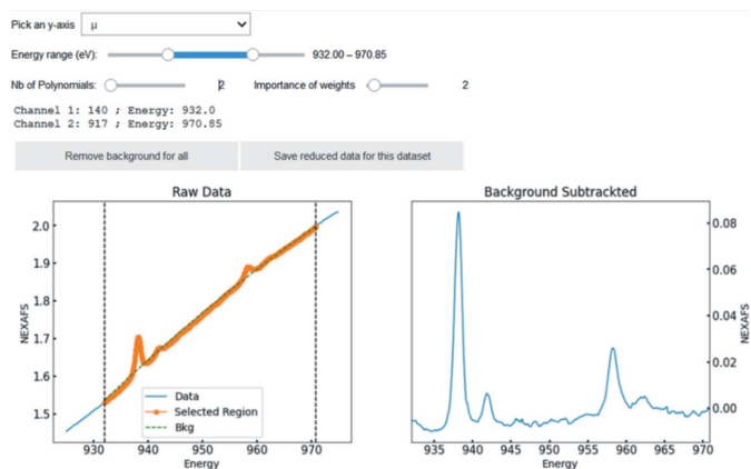
Figure 11 Application of the Chebyshev polynomials method to remove the background from a representative region of a NEXAFS spectrum, corresponding to the Cu L -edge (orange points, left panel), containing both the L_2 - and L_3 -edges. The degree N of the polynomials and the importance of weights can be changed by sliders and directly control the shape of the background curve computed via the NumPy class method Chebyshev.fit function.
