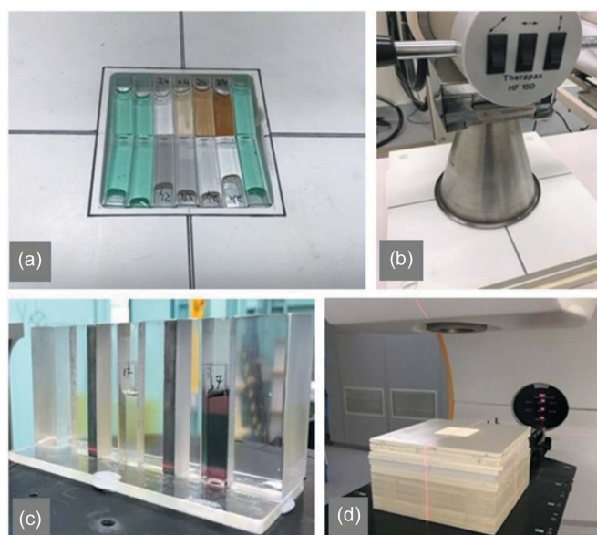
Figure 3 (a) Solid water phantom enclosing PRESAGE cuvettes, (b) setup for SXRT irradiations, (c) PRESAGE cuvettes in a Perspex phantom and mounted on the sample stage goniometer on the IMBL, (d) setup for linac irradiations.
