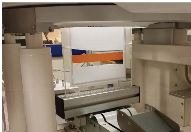
Figure 4 Photograph of the under-table beam profile measurement setup, using a flat piece of radiochromic film positioned at the isocenter, normal to the incident beam.
