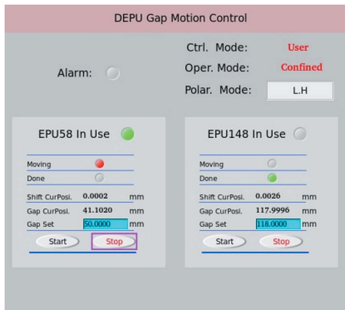
Figure 6 Control interface for the users of the DREAMLINE beamline undulators.
