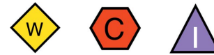
Figure 2 Indicators used by Karabo for, from left to right, warning, alarm and interlock alarm types.
