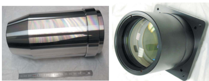
Figure 2 Macroscope optical components: front infinity corrected objective (left) and tube lens (right).
