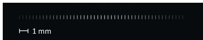
Figure 4 Image of the 20 mm × 520 µm parallel array of microbeams obtained with the FReLoN camera.
