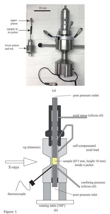
Main body of the HADES rig. (a) Sample assembly and body of the rig. (b) Cross section of the rig.
