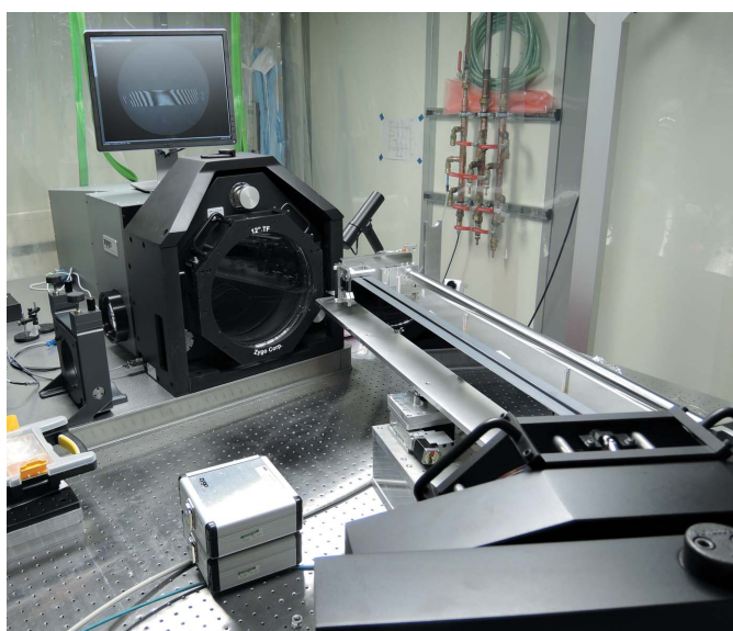
Figure 2 Photograph of the mechanical bendable mirror placed between two auxiliary optical flats, creating an optical cavity in an angled incidence setup. The screen above the beam expander shows an image of the interference fringes.
