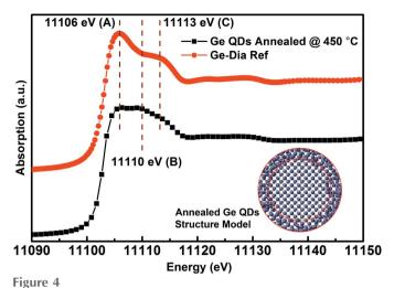
Position of features in the XANES spectra of annealed Ge QDs and the diamond-type Ge reference. The feature in the middle cannot be observed in the reference XANES spectrum. The positions were obtained by taking the derivatives of the XANES spectra. The inset is an illustration of the proposed core-shell model for annealed Ge QDs.
