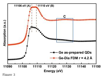
Comparison of experimental XANES spectra of as-prepared Ge QDs with simulation, for which only the first two shells are included in the calculation cluster (radius r = 4.2 Å) using FDM mode.
