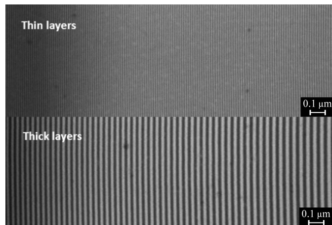
Figure 1 SEM images of the cross section of \text{WSi}_2/\text{Si} multilayers. White layers are \text{WSi}_2 ; black layers are Si.
