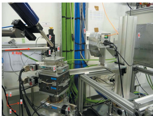
Figure 7 Photograph of the experimental set-up. The beam comes from the left. Main elements are numbered: (1) sample; (2) translation-rotation stage; (3) cryostream; (4) beamstop; (5) XPAD3S-CdTe (in position for acquisition); (6) the MAR345 protected by a lead screen and displaced from the acquisition position during the XPAD measurements.
