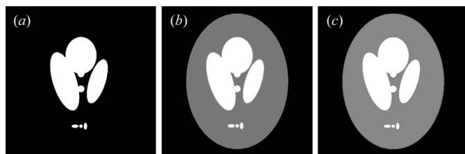
Figure 2 Numerical phantom with 1024 \times 1024 pixels. (a) Zn distribution. (b) Attenuation map at the incident X-ray energy. (c) Attenuation map at the Zn characteristic K\alpha X-ray energy.
