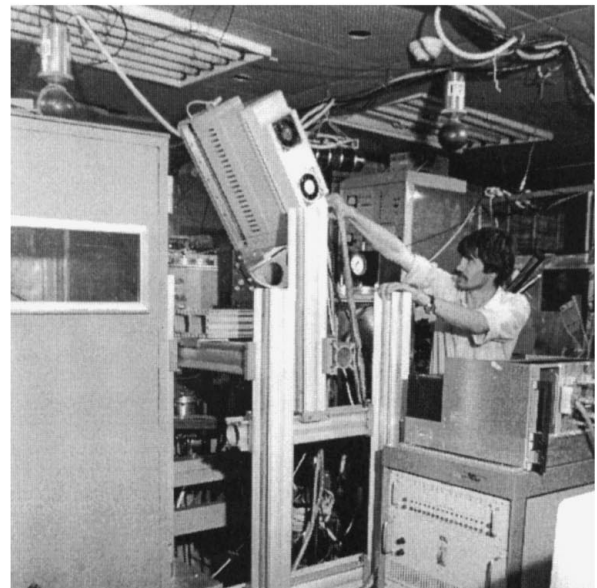
Figure 4 The OD-160 detector: (a) schematic diagram of the detector, (b) a photograph of one section of the detector with an aperture of 16° installed at VEPP-3 synchrotron radiation beamline 2-b.
