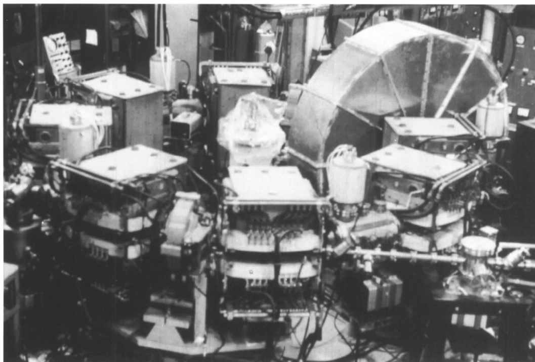
Figure 1 Tantalus. Seven of the eight bending magnets can be seen. The ‘disk’ on the right is the r.f. cavity. The University of Chicago’s focusing-mirror chamber is in the foreground.
