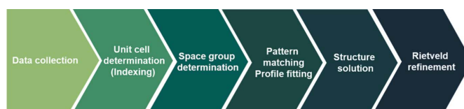
Figure 3 Structure determination from the powder X-ray diffraction (PXRD) procedure.
