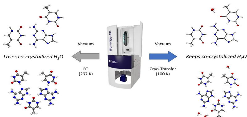
Figure 1 Two examples illustrating cryo-transfer is important: (left) structures measured at ambient temperature and vacuum, and (right) using a cryo-transfer station at 100 K.
