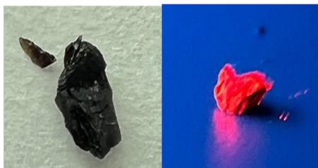
Figure 1: Light emission property of 2,6-Diaminopyridine perovskite under short wavelength UV light
