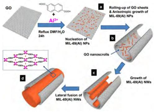
Formation mechanism of single crystal MIL69(AI) NW
