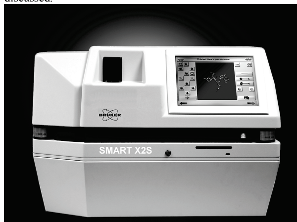
Figure 1: SMART X2S table top SC-XRD solution.
